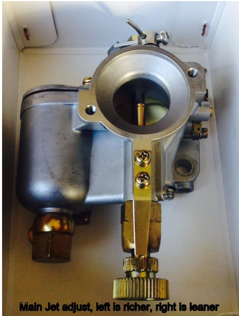
Figure13. A typical Yamato carburetor. Main jet adjustment is performed with the large knob. IN is leaner, OUT is richer.
