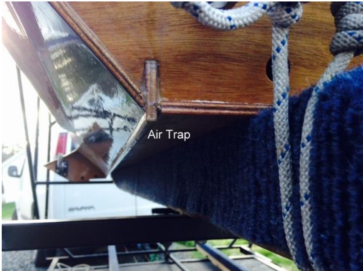
Figure 9. The rear view of a typical left airtrap. This one is about ¼ inch deep at the transom.
